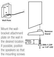
(not included; use size #8) may be installed directly into a wooden wall stud. If that is not possible, use optional wall anchors that are rated to support at least twenty-five pounds. The customer is responsible for proper selection and use of mounting hardware, available through hardware stores, to properly and safely wall-mount the speakers.
